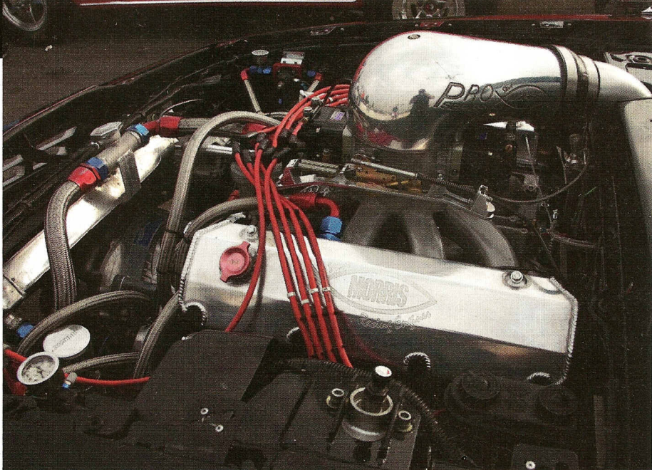
> Above: Steve Morris Racing Engines built the big-inch Ford to make ridiculous power with a direct-drive ProCharger F-3 blower, which exhales through tubing that leads to a huge water-to-air intercooler and is then redirected into the CSU-prepped Dominator carburetor. The T-bird almost didn't make it past the drive, as Jim saw 300-degree water temps on his data logger in Memphis' traffic. It didn't seem to hurt anything, though. HRM
